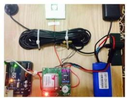
Fig. 3: Experimental Setup of Proposed System
