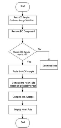
Fig. 2: Flowchart chart of sensor data processing
